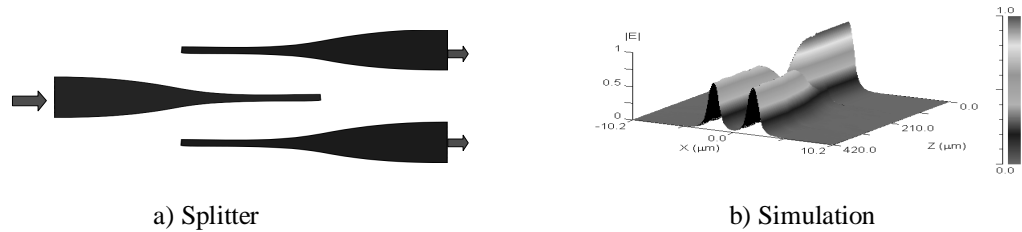
Fig. 1. The picture of optical splitter of coupled tapered waveguides and splitting result of BPM simulation
